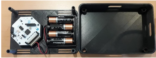
Figure 10 OpenBCI Cyton board and accessories for monitoring biosignals.
