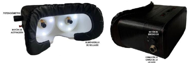
Figure 2. Electronic Device for Measuring Sclera Colouring [15].
