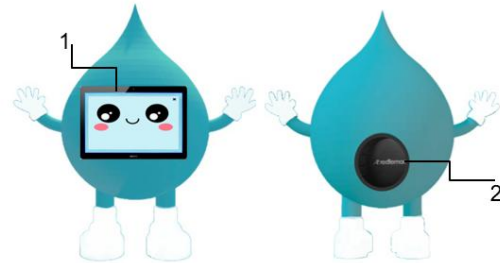
Figure 4. Arroyuelo: serious game embedded in a 3D droplet to teach water scarcity concepts in rural communities, 1) embedded tablet for visual feedback, 2) circular speaker for auditory feedback
