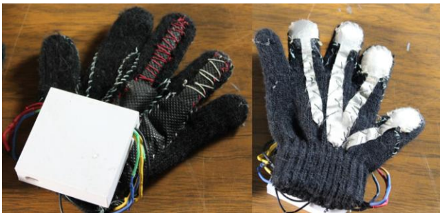
Figure 6. Gloves with flex and touch sensors relocated.
