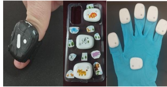
Figure 2. Shows different interaction devices (ring, smartphone case, glove) to test the sensations of the vibrotactile patterns.
